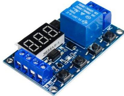
It is 6-30V 1-Channel Delay Power Relay Module with Onboard Adjustable Timing Cycle Switches with Digital LED display It is mostly used in Home Automation Delay Timer Control Switch Module Timer Controller. The Module operates at Operating voltage range of 6-30V, also it supports micro USB 5.0V power supply. Output capability: Can control the device within DC 30V 5A or AC 220V 5A. It can be applied to many fields as there is a wide range of application.
